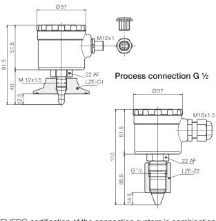
EHEDG certification of the connection system in combination with weld-in sleeve LZE (see page 191-198)
